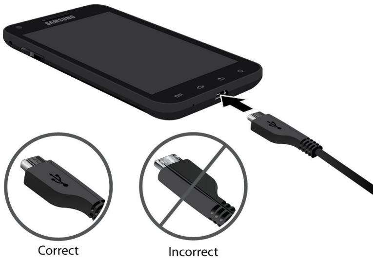
3. Plug the AC adapter into an electrical outlet. Fully charging a battery may take up to three hours.
